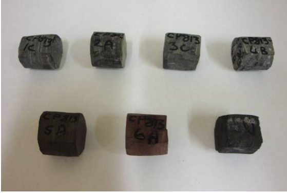
Figure 3. Photo of samples CP813-1C – shale, CP813-2C – shale with dropstones, CP813-3C – mudstone, CP813-4B – tillite, CP813-5A – hematite, CP813-6A – lava, CP813-7C – Mn-ore
