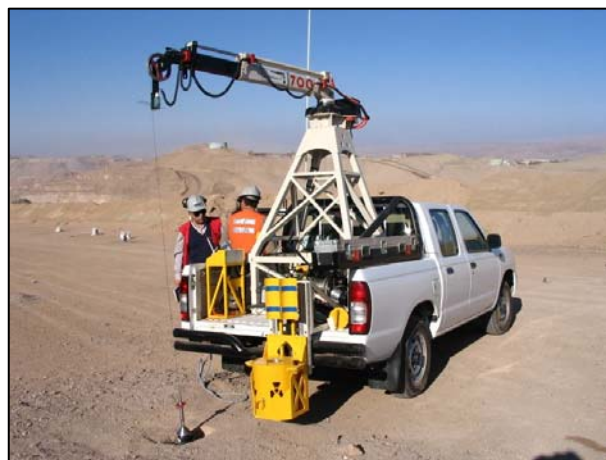
Figure 8: Design of SIROLOG logging system for on-mine operations, Chile
