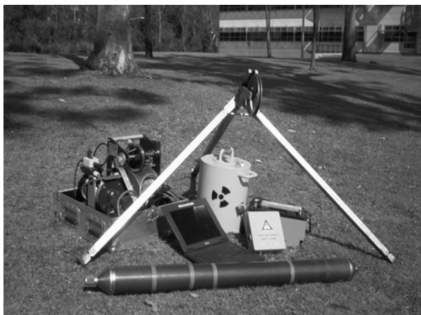
Figure 2: Components of the SIROLOG PGNAA portable logging system
