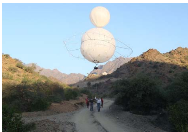
Figure 1. TDEM balloon in operation in Yemen. The loops are about 5m above the surface.
