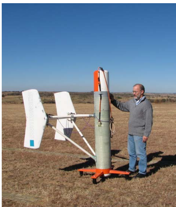
Figure 4. Predecessor towbird which proved not to be very aerodynamic in the wind tunnel. L. Polomé for scale.
