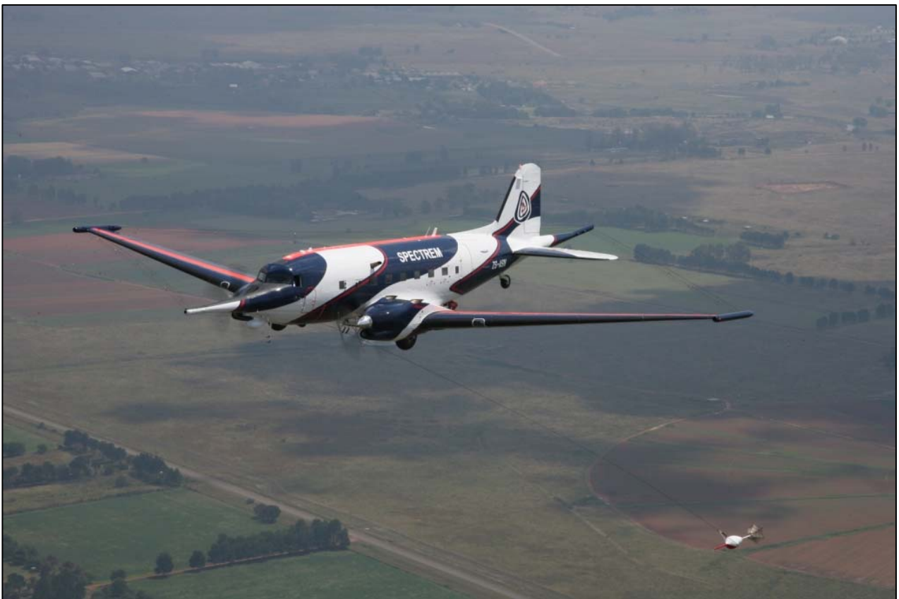
Figure 2. Spectrem 2000, with towed EM receiver
