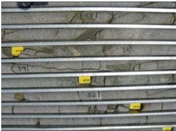
Figure 5. Core photo of upper hazardous zone in BH1
