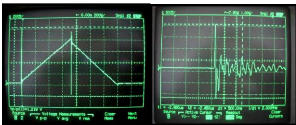
Figure 3: High frequency (2Mhz+) transmitter switching noise as seen on an oscilloscope.
