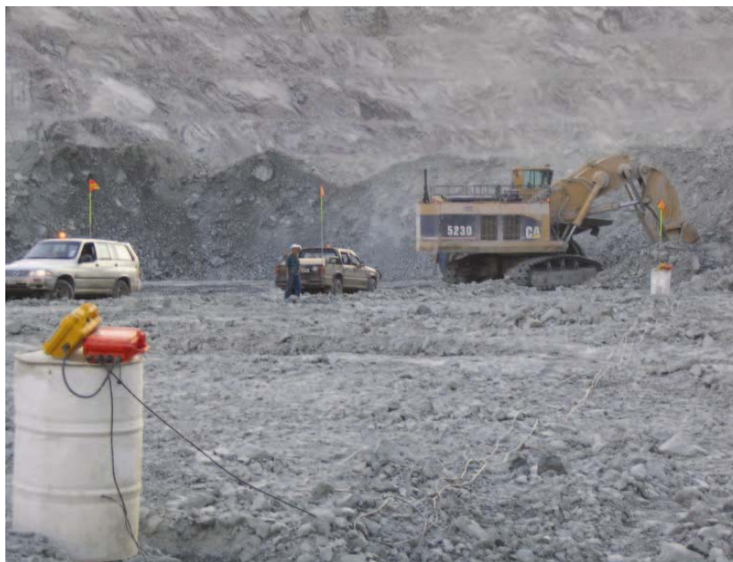
Figure 2: DAS survey collecting DCIP and MT data in active open pit mine. Receiver nodes shown with 50 m spacing in this application mapping side walls in kimberlite. Photo taken in Venetia Diamond Mine, South Africa.
